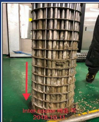
As a result of comparison before and after the operation of the cooling tower eliminator in the bottled water plant in Korea, it can be seen that the scale of the surface was removed 35 days after operation
