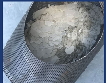
Scale collected in the inner strainer after 15days of operation.
